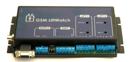
The GSM Lift Watch provides communication between a lift cabin and hotline service (first aid) via GSM network. After pressing the alarm button on the control panel in the lift cabin the GSM Lift Watch automatically dials up a preprogrammed number (up to 8) and establishes a connection with hotline service (first aid).
